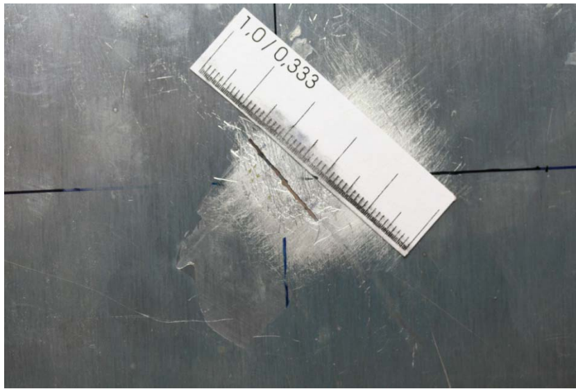
Fig. 6: Crack length of panel 01
